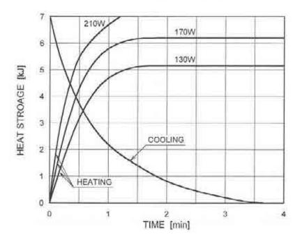
Heating/cooling curves of the TOSHIBA DG-073B-DC
